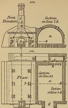
burnt; these holes are closed up whilst the firing is proceeded with; fff, sight-holes to watch progress of the burning; gg, firing holes;  $\hbar\hbar$  and jj, stoke-holes for stoking the fires and breaking
